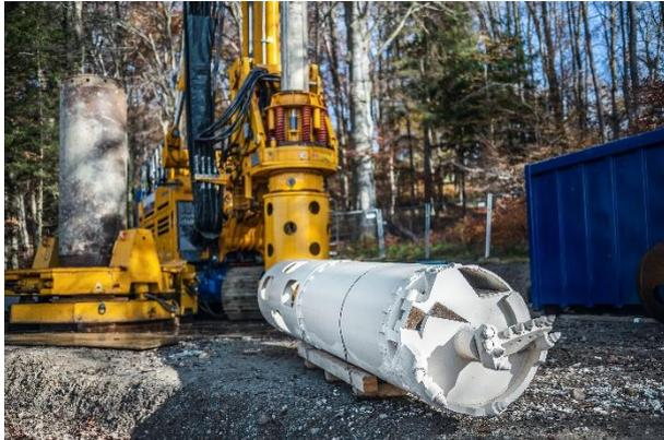
(2) A specially developed KBF-K drilling bucket with guide casing was used for the project.
