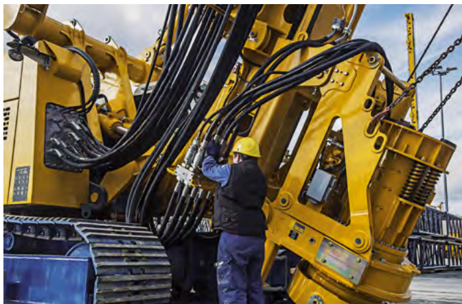
Rigging position for connecting of hydraulic hoses
