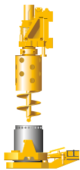
Cased Kelly drilling Casing installation with casing oscillator (additional power pack required)
