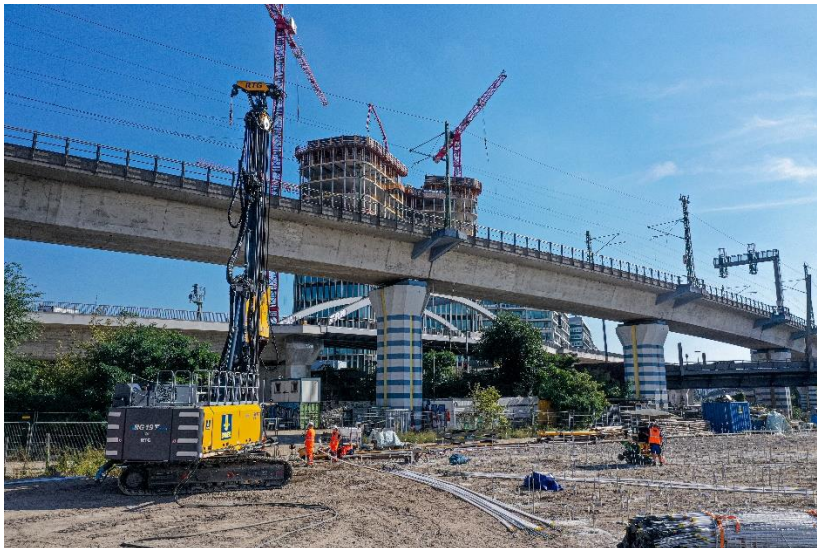
(2) Low noise, reduced CO 2 emissions: The innovative hybrid drive combines the performance level of a 430-kW diesel engine with an 88-kW electric motor.
