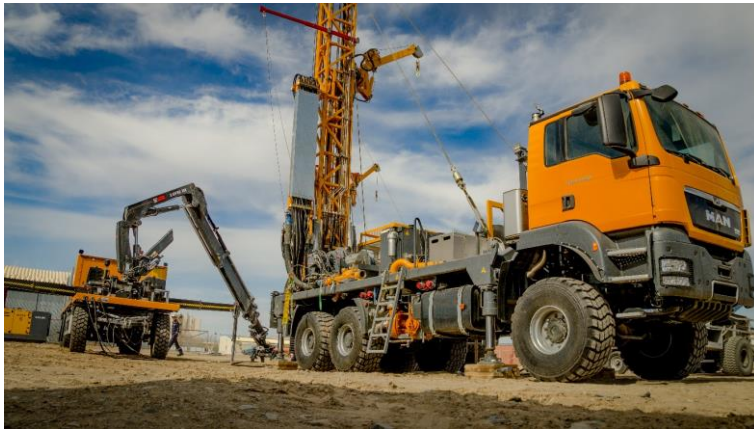
(2) RB 65 with special equipment for operation in the desert of Kazakhstan with automated drill string handling system
