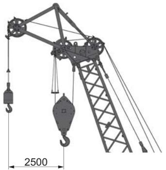
The optional auxiliary jib is designed for single strand operation up to max. 35 t. Conditions for lifting operations apply for rated loads.
