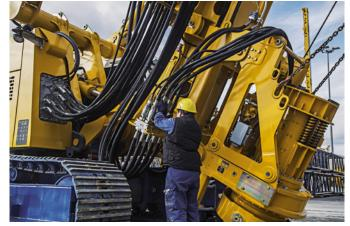
Rigging position for connecting of hydraulic hoses
