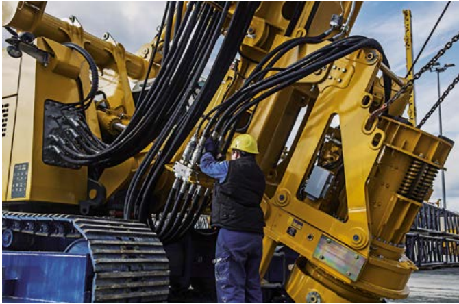
Rigging position for connecting of hydraulic hoses
