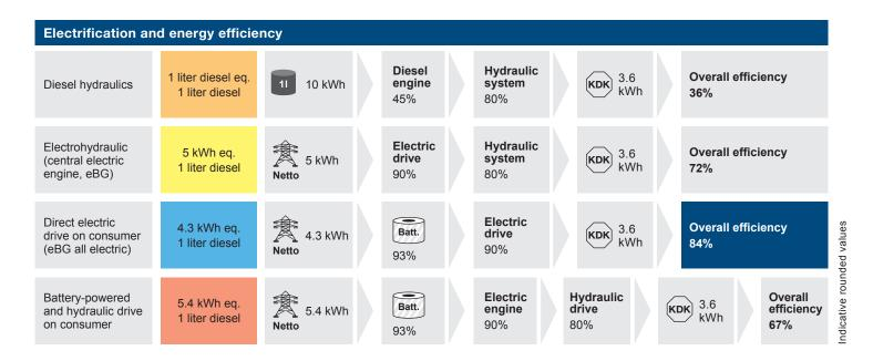
The implemented primary energy is utilized to maximum capacity. This is reflected both in the energy consumption as well as in the runtimes of the drilling rig (8 h operating time with average kelly drilling). As a result, the eBG 33 H
