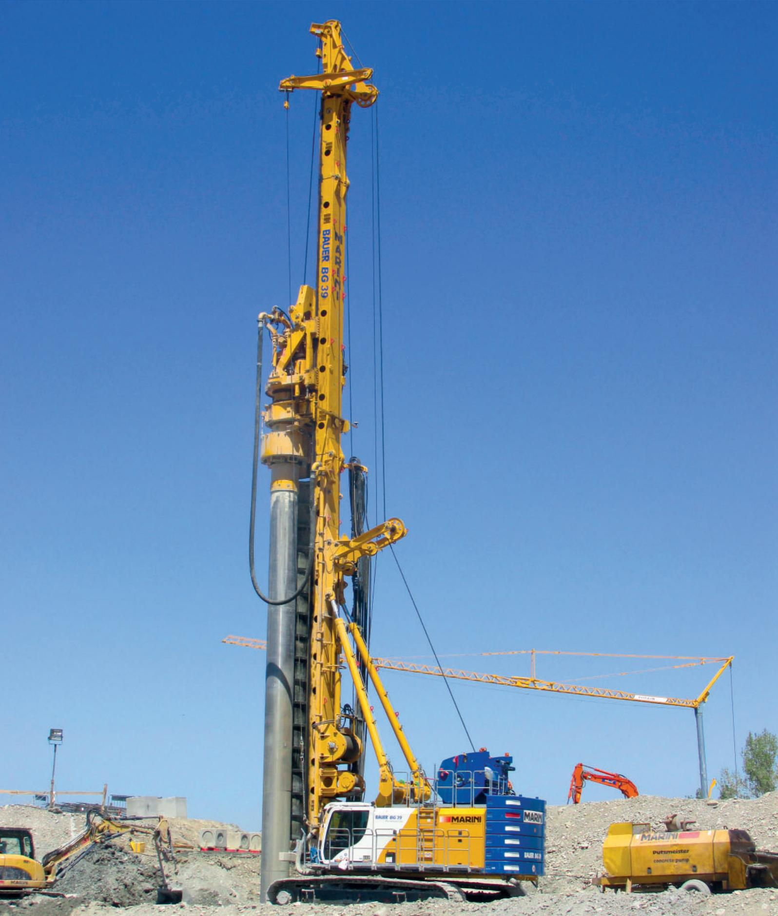
By using long continuous flight augers (CFAs), which are drilled into the ground in one piece, the drilling performance can be increased significantly. In contrast to the CFA technique, the CCFA technique is carried out by drilling a casing string simultaneously with the continuous auger into the ground.
