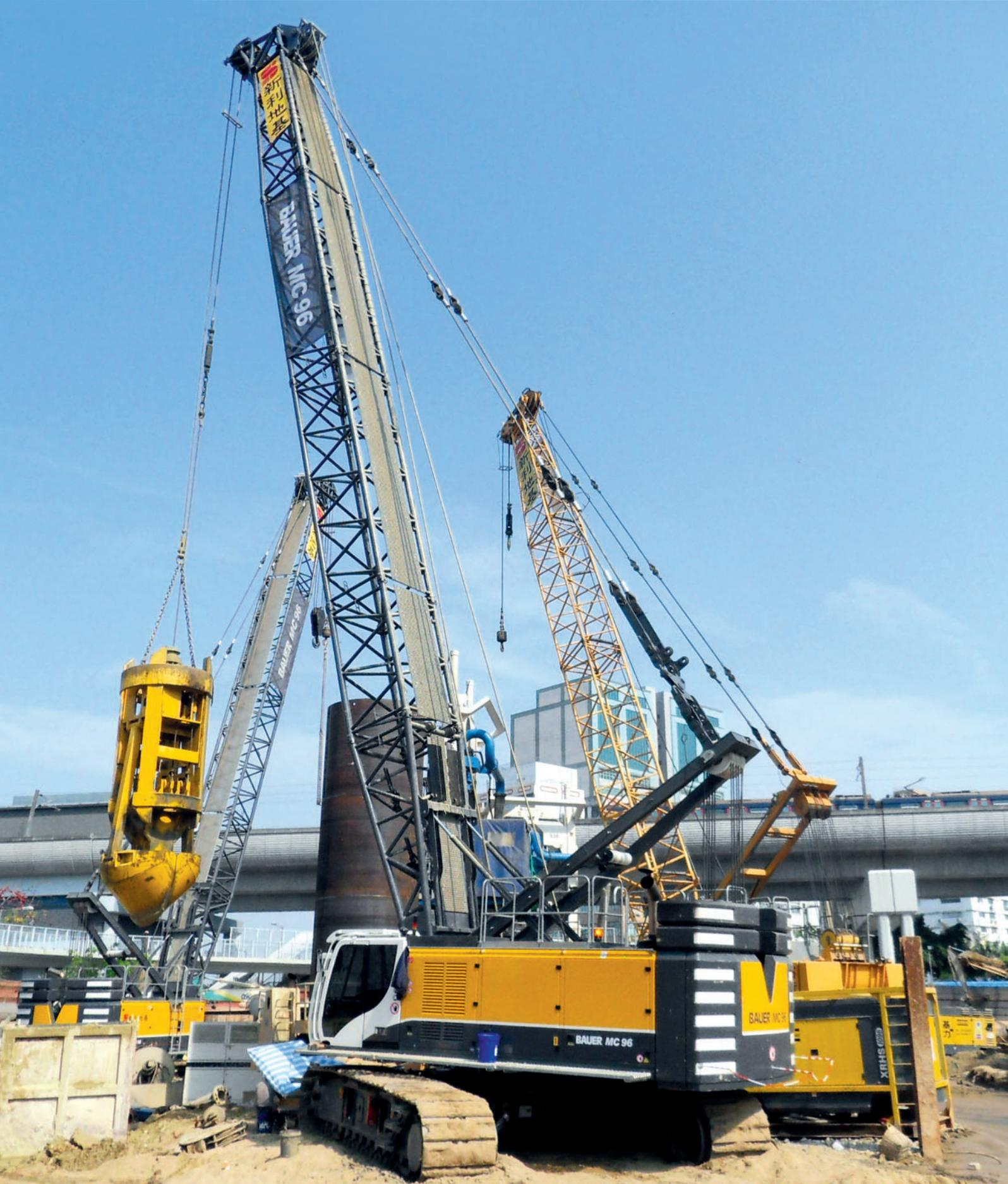
**The duty-cycle cranes can be used for multi-purpose applications in specialist foundation engineering:**
