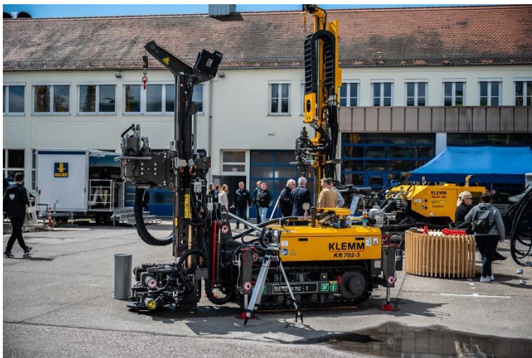
(5) The KR 702-3 offers impressive features including a new hydraulic and electric control system.
