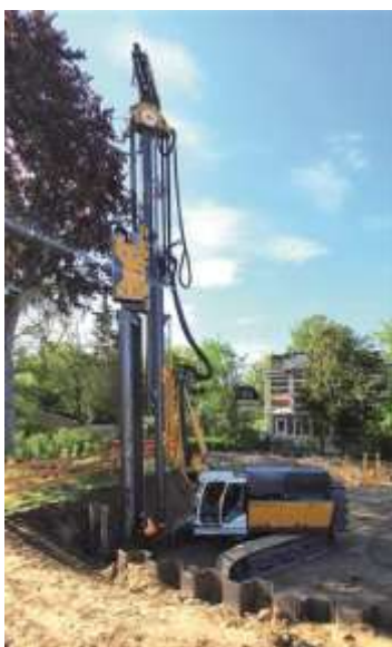
(1) RG 19T with integrated sheet pile assistant at a project in Berlin, Germany
