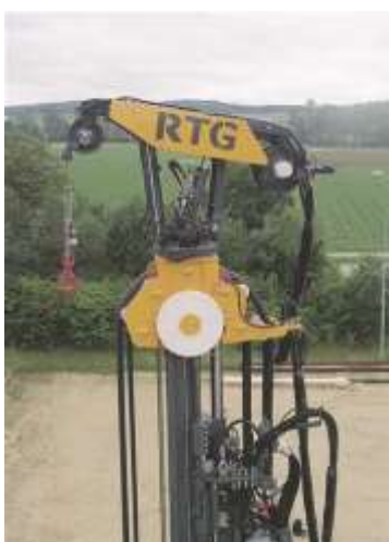
(4) The new auxiliary winch
