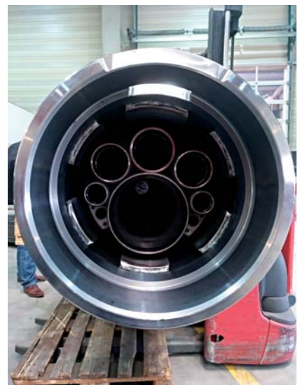
Uranium mining, Canada HPRC mining pipe section with process lines
