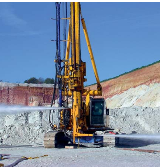
Kaolin mine, Germany High pressure jet mining with foldable nozzle arms
