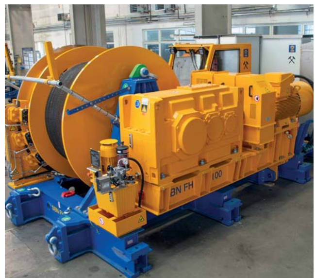
Mining hoist Compact mining hoist for working service and rescue
