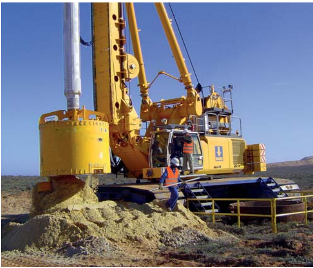
DeBeers Kleinzee Mine, South Africa Sampling of alluvial diamonds up to 100 m depth with BG 48, dia. 2.5 m
