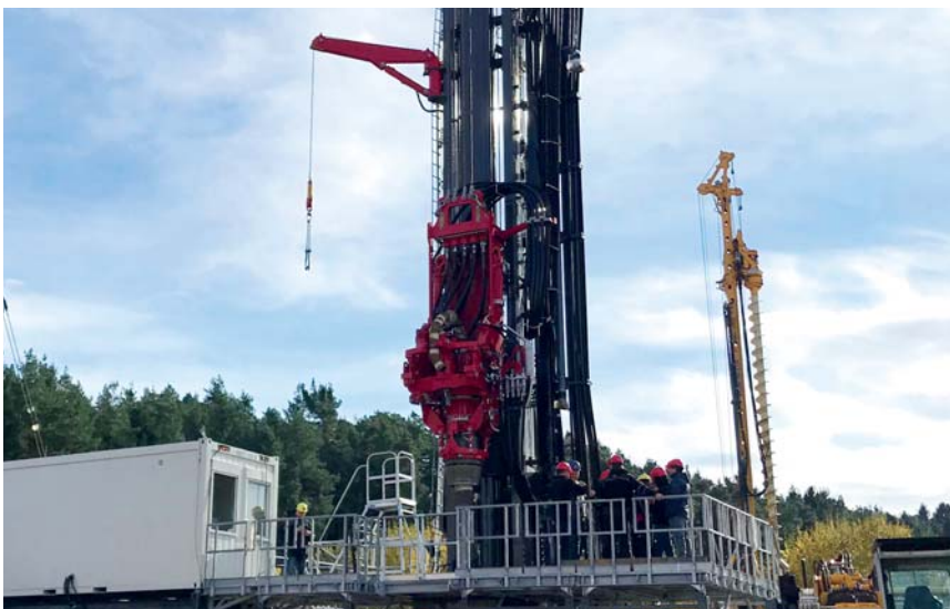
Uranium mining, Canada HPRC system mounted on RB-T 100 base machine
