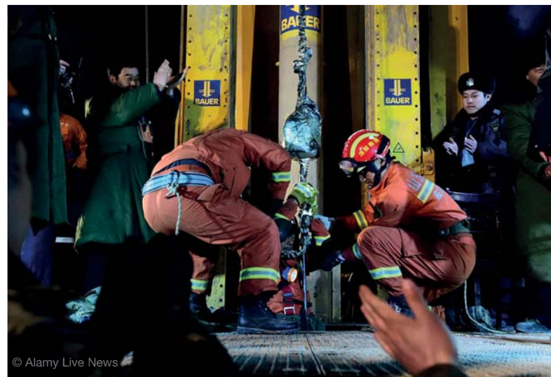
Pyngi Mine, Shandong Province, China 4 miners had been rescued via a 711 mm drilled hole to 226 m, after 36 days being trapped underground
