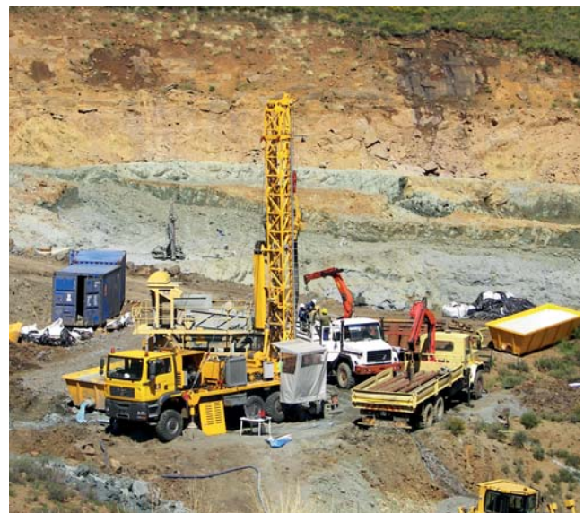
Liqhobong Kimberlite Mine, Lesotho 17 ½" RC bulk sampling
