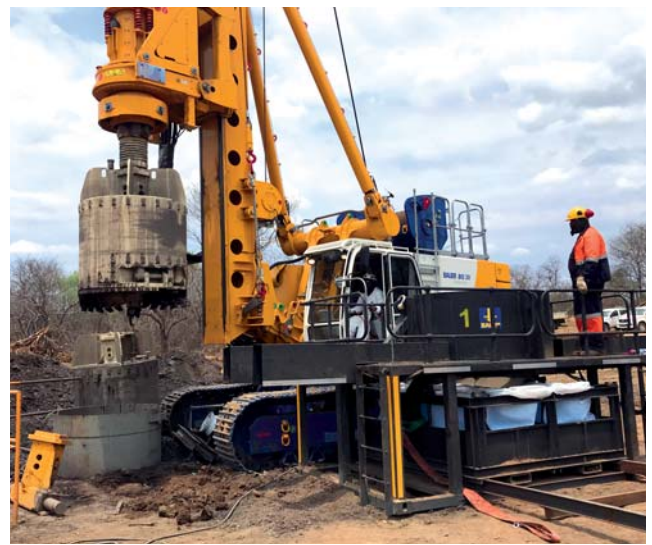
Vale coal mine, Mozambique Coal grade control, diameter 1.5 m to 80 m depth with BG system
