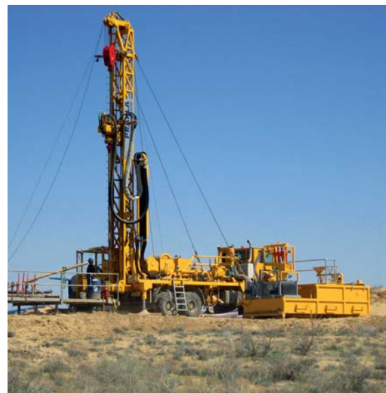
Uranium mine, Kazakhstan Installation of production wells for insitu leaching
