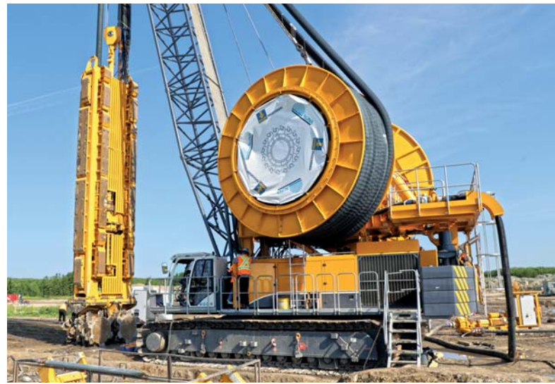
FalCon Project, Saskatchewan, Canada Cutter bulk sampling to 250 m depth
