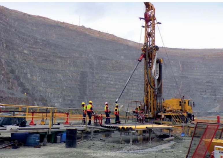
Jwaneng Diamond Mine, Botswana 5 ½" wireline core drilling
