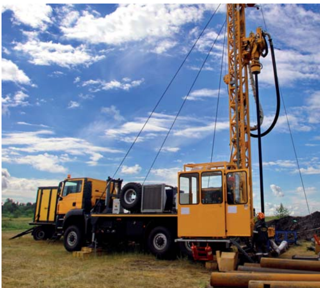
Coal mine, Kuzbass Region, Russia Degasification of coal layers prior to underground mining
