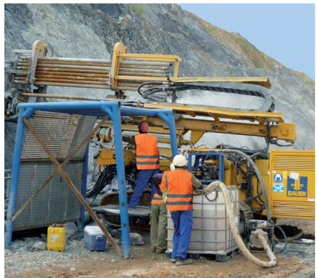
Newmont Gold Mine, Ghana 120 m long horizontal depressurization wells
